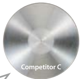
The finished surface is clouded
