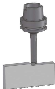
Milling of the jaw to the required height
