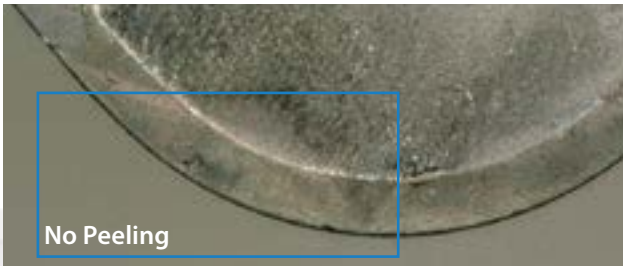
Cutting conditions : Vc = 150 m/min, ap = 0.2 mm, f = 0.2 mm/rev, Dry Workpiece : SCM 415® (In-house evaluation)
