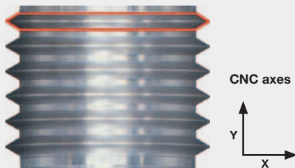
Creation of the thread with thread milling
