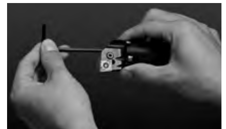
3. Tighten 3 bolts to attach the head
