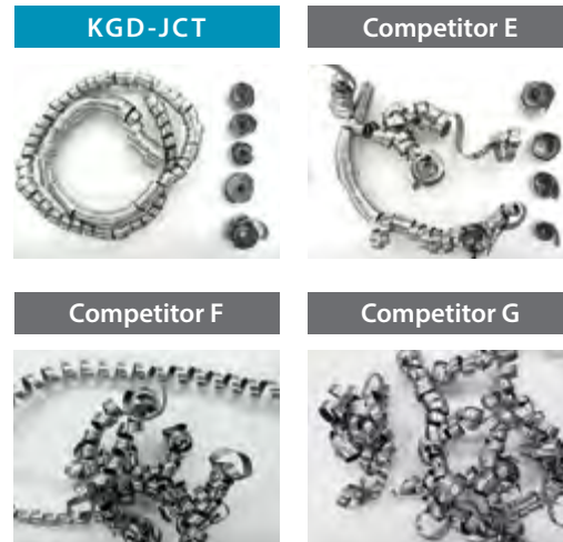
Cutting Conditions : Vc = 150 m/min, d = 8mm, f = 0.05 mm/rev, Wet Edge Width 4 mm Workpiece Material : 15CrMo4 Grooving
