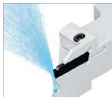
Effective cooling of the cutting edge
