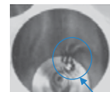
Chips are adhering to the bottom when drilling stops.
