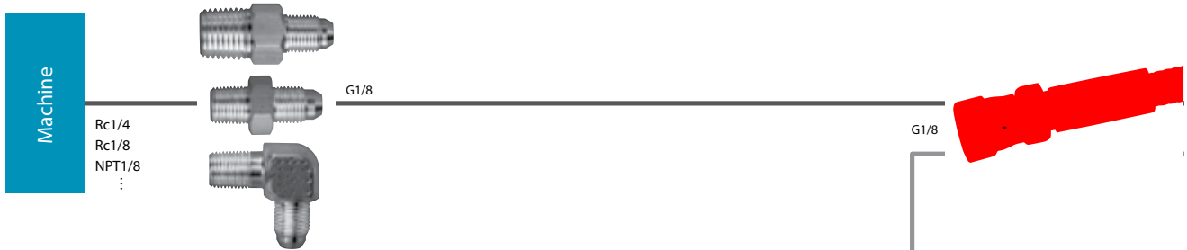
With coupling (Pump pressure: Up to 7.5 MPa)
