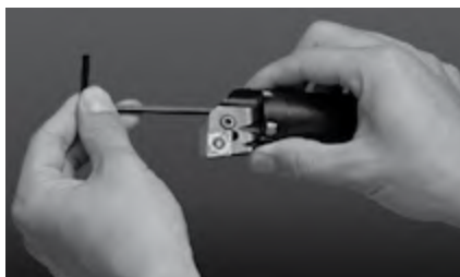
2. Tighten 3 bolts to attach the head
