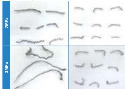
f = 0.05 mm/rev f = 0.15 mm/rev f = 0.05 mm/rev f = 0.15 mm/rev Cutting conditions: Vc = 150 m/min, ap = 0.5 mm, Wet, CNMG120408 type Workpiece material: 15CrMo4 External turning
