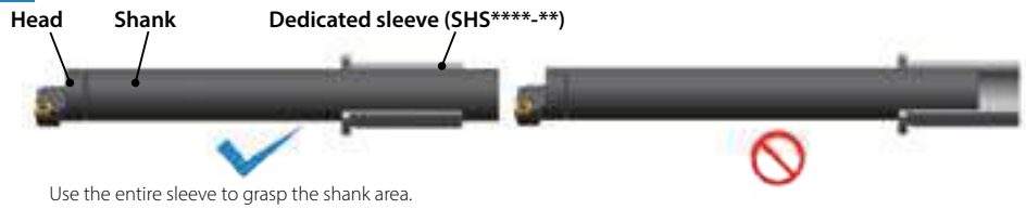
Use the entire sleeve to grasp the shank area.
