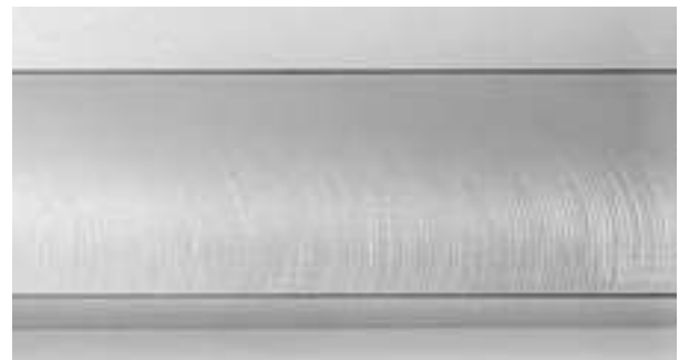
Excellent surface finish with low workpiece clamping rigidity
