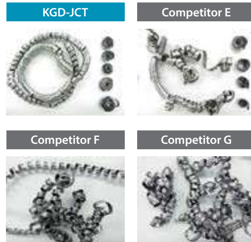
Cutting Conditions : V_c = 150 \text{ m/min} , d = 8 \text{ mm} , f = 0.05 \text{ mm/rev} , Wet Edge Width 4 mm Workpiece Material : 15CrMo4 Grooving
