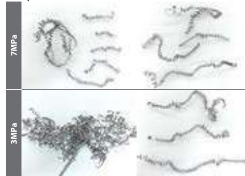
f = 0.05 mm/rev f = 0.15 mm/rev f = 0.05 mm/rev f = 0.15 mm/rev Cutting conditions: Vc = 150 m/min, ap = 0.5 mm, Wet, CNMG120408 type Workpiece material: 15CrMo4 External turning
