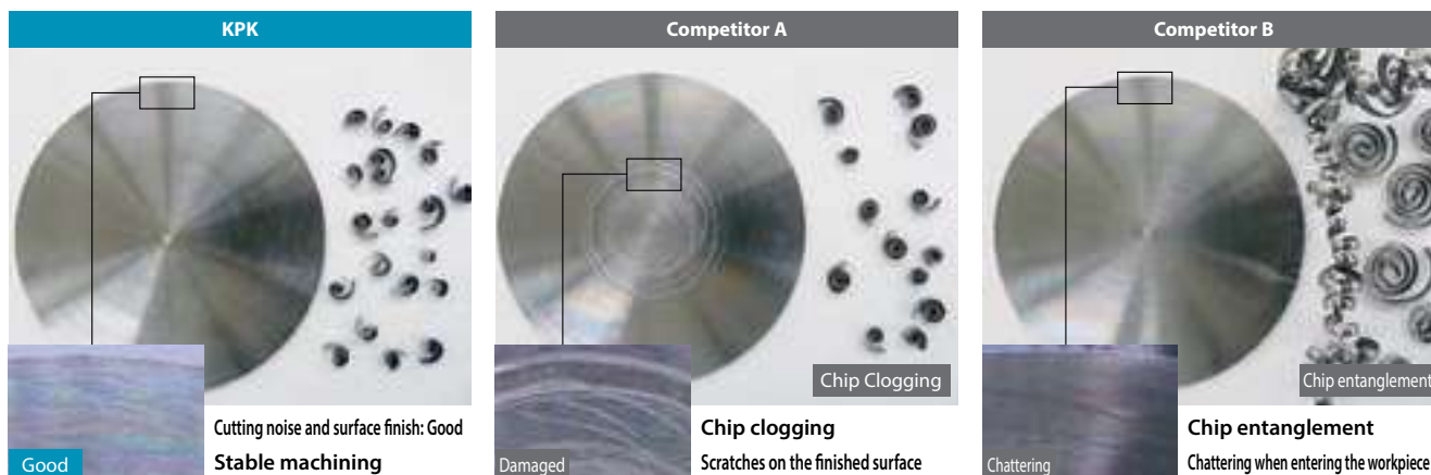
Cutting performance comparison (Internal evaluation)
