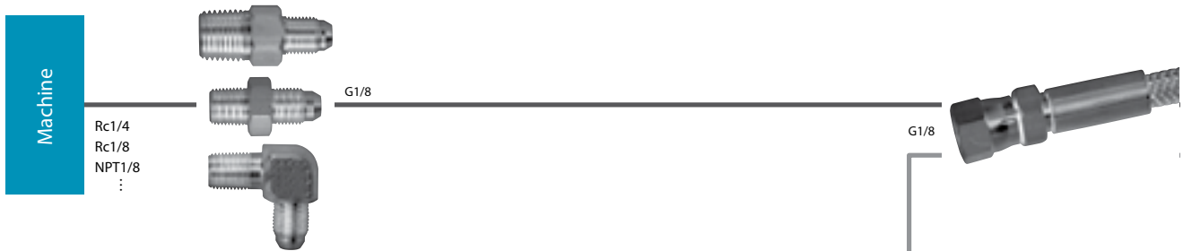
With coupling (Pump pressure: Up to 7.5 MPa)
