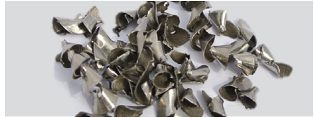
Cutting conditions: workpiece: stainless steel 316L, VC = 60 mm, f = 0.16 mm/rev.
