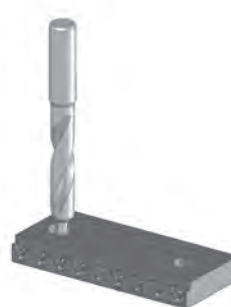
Drilling of the jaw with the correct distance of the holes
