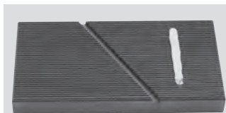
Apply grinding compound (corn 320) near the outer edge.
